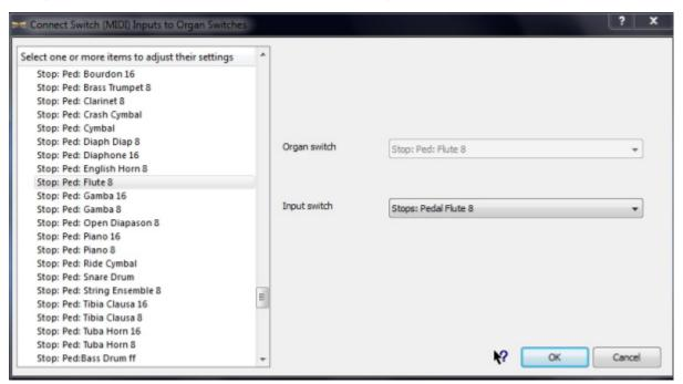
You can now connect all couplers, stops and switches that the sample set provides to your newly defined MIDI switches, simply matching name for name. As in the example above, the Pedal Flute 8' stop on the organ is connected to the MIDI switch Pedal Flute 8 that was defined for it. EVERY other switch can be connected in this way - just match like for like.
